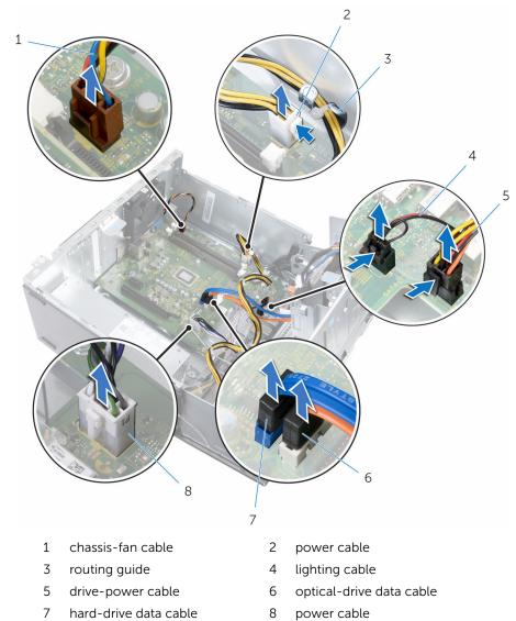
2 Note the routing and move the cables away from the system board.
