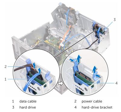
4 Spread apart the hard-drive bracket from one edge and lift the hard drive up.
