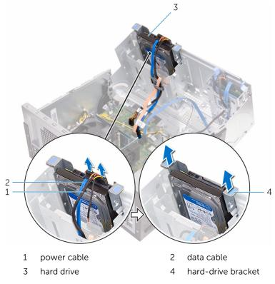
**5** Remove the screws that secure the hard-drive bracket to the hard drive.
